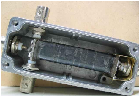
Photo 5. Balun inserted in box. BNC connectors were put in first then balun soldered at Reference/Unknown end first. Balun then hinges at this point and can be swung down to mate with the brass shim and the receiver BNC.
